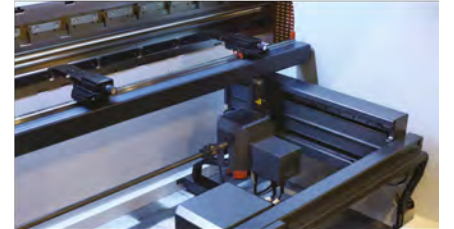
İki eksen arka dayama (X-R) Two axis backgauge (X-R)
