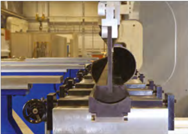
Abkant Pres Tandem Asimetrik 8100/4100 mm x 800/440 ton Press Brake Tandem Asymmetric 8100/4100 mm x 800/440 tons
