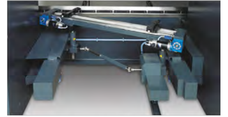
Beş eksen arka dayama (X1-R2-R-Z1-Z2) Five axis backgauge (X1-R2-R-Z1-Z2)
