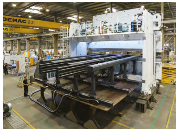
Abkant Pres 9100 mm x 3000 ton Press Brake 9100 mm x 3000 tons
