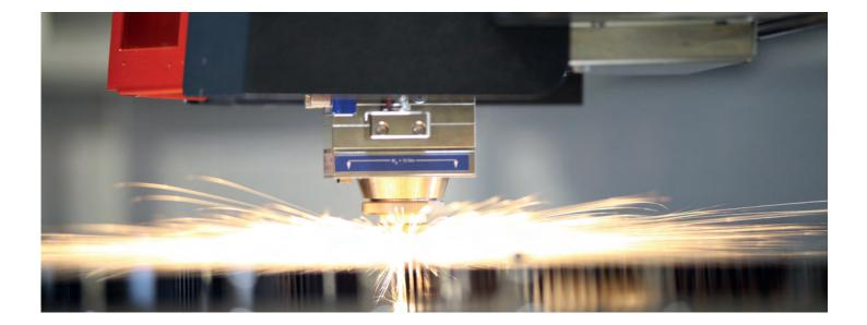
BLS Series Fiber Laser Cutting Machines cover a wide range of industrial applications. Manufactured as "All in One Box" Design structure, the BLS has built in Resonator, Chiller with dual motorized table. A range of fiber power sources starting from 500W to 2500 W are Available. The "BLS" uses new generation high performance linear axis system with high performance rack and high performance class pinion.
